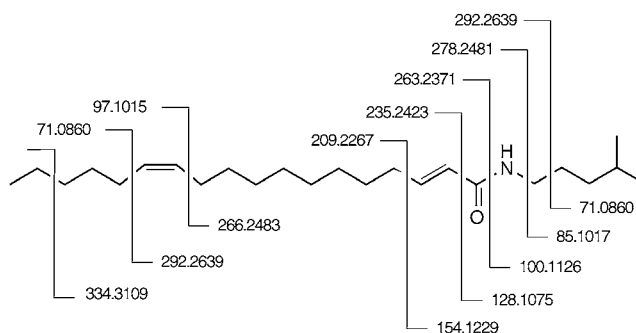
Fig. 2. Observed HR-EI-MS fragments (in m/z ) of pipzurine ( 2 )
